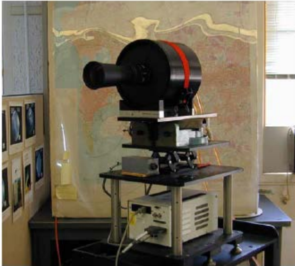
Figure 9-2. MSI sensor head, with zoom lens and 16-bit digital CCD camera
